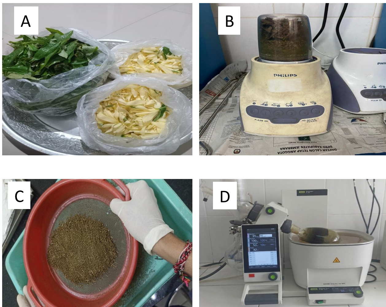
Figure 1. Processing and extraction of plant materials: (A) fresh plant materials, (B) drying process, (C) grinding into powder, and (D) extraction using a rotary evaporator.
